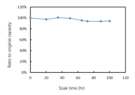
After being soaked in 0.1 M NaOH for 100 hours, the capacity of GP-ProA resin was 94% of the original capacity, with a small decrease. In actual use, the CIP cleaning time of each cycle is generally  $\leq$ 0.5 h, and 100 hours of soaking time is equivalent to 200 CIP cycles.
